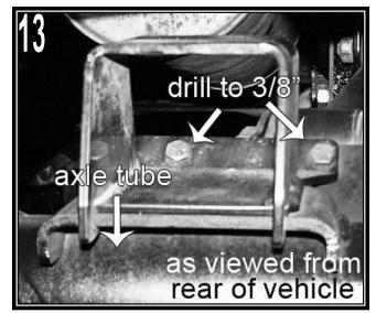
using the holes in the bracket as a template, drill two holes through the factory pad for the 3/8" mounting hardware. Insert the supplied 3/8" x 1" bolts (installed from top), flat washers (on nut side), and Nyloc nuts. Tighten (30).
