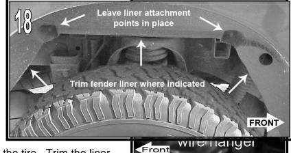
have to be trimmed to minimize contact to the tire. Trim the liner horizontally on the angled face above the area of contact. Leave
